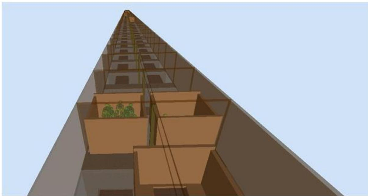
Figure 8: Simulation of Skytrak depicting Multiple Cars in Each Shaft and Transfer of Cars Below Main Lobby
