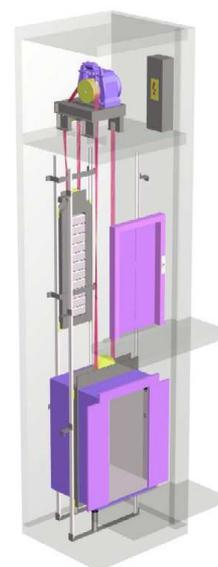
**Figure 1** shows typical traction lift with counterweight
