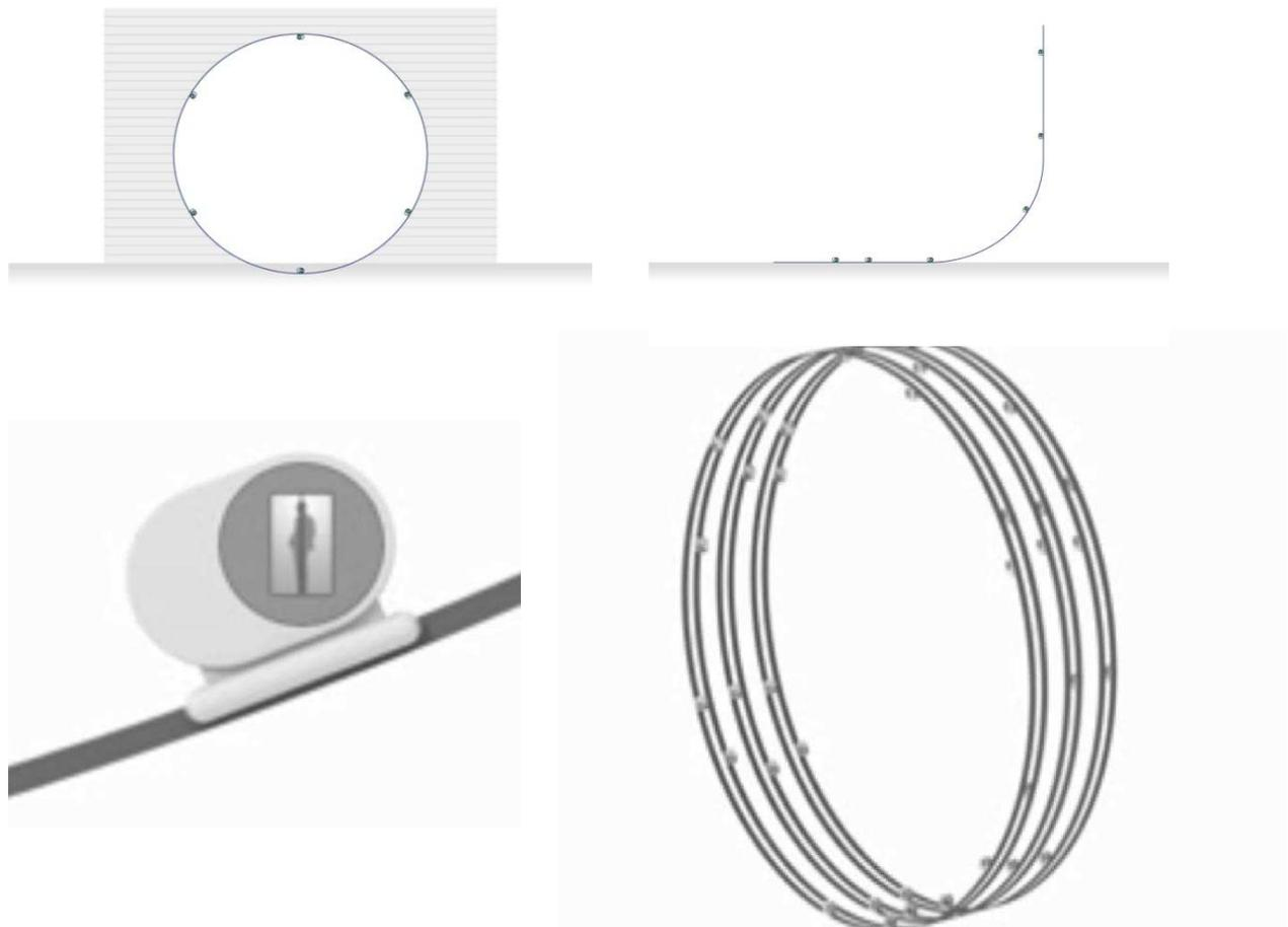
**Figure 9** New shapes of buildings are now possible using the “Skytrak” circular transportation solution operating on 360 degree oriented tracks with multiple cabins
