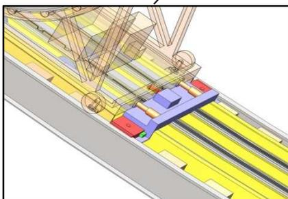
After this controlled deceleration the cabin then rolls back, with the retarders reconnected with their tuning capacitors, at controlled speed to rejoin the main drive assembly and thence to continue its safe descent downwards at low speed to the nearest floor served or the lowest part of the track system for release of passengers
