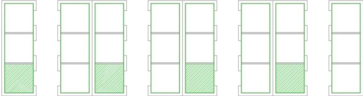
Supposing one passenger lift @ 1600kg at 6.0m/s appeared in one shaft travelling “up” every 30s. At the main lobby we would have a revised footprint of lift shafts and lobbies that looked like this:
