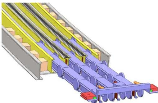
**Figure 3** shows the main drive moving magnet assembly (blue) with articulated sections, guide wheels and brakes (red)
