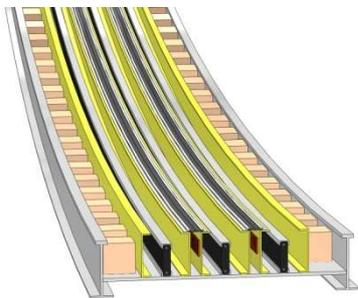
**Figure 2** shows the main track structure comprising three double sided linear motor stator sections (black), twin magnet tracks for not only safety retarding under gravity and on-board power generation but importantly deceleration control during emergency “up” stopping. Track side power switching devices are also shown
